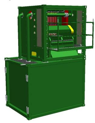
The pump tank module houses a Svedala 150x100 centrifugal pump with 30kW overhead motor used to supply fluid to the hydrocyclones. Also mounted in the unit is another Svedala 150x100 pump with 30kW motor. This is used to transfer the processed fluid away from the machine. Both motors for these pumps have star delta starting. The pump tank module also has a stores compartment with a small compressor and electrical control equipment, mounted within that compartment.
